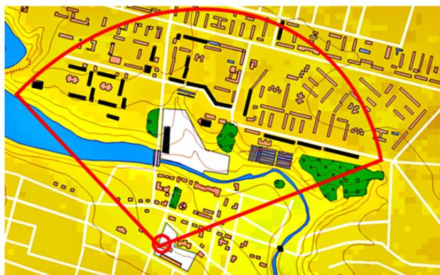
FIGURE 4: The map of city area. The red circle corresponds to the radar location while the red circuit illustrates scan range. The houses are included in 3D-scene are marked black.
